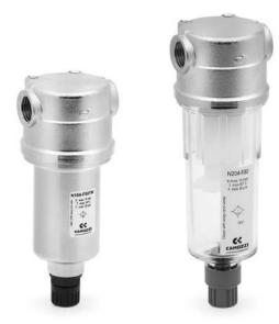
Series N filters are available with G1/8 and G1/4 gas ports. The models are available with 3 different filtering elements: 25, 5, 0.01 $\mu$ m and actived carbon.
