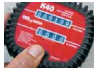
Mechanical counter with total-partial resetting.
